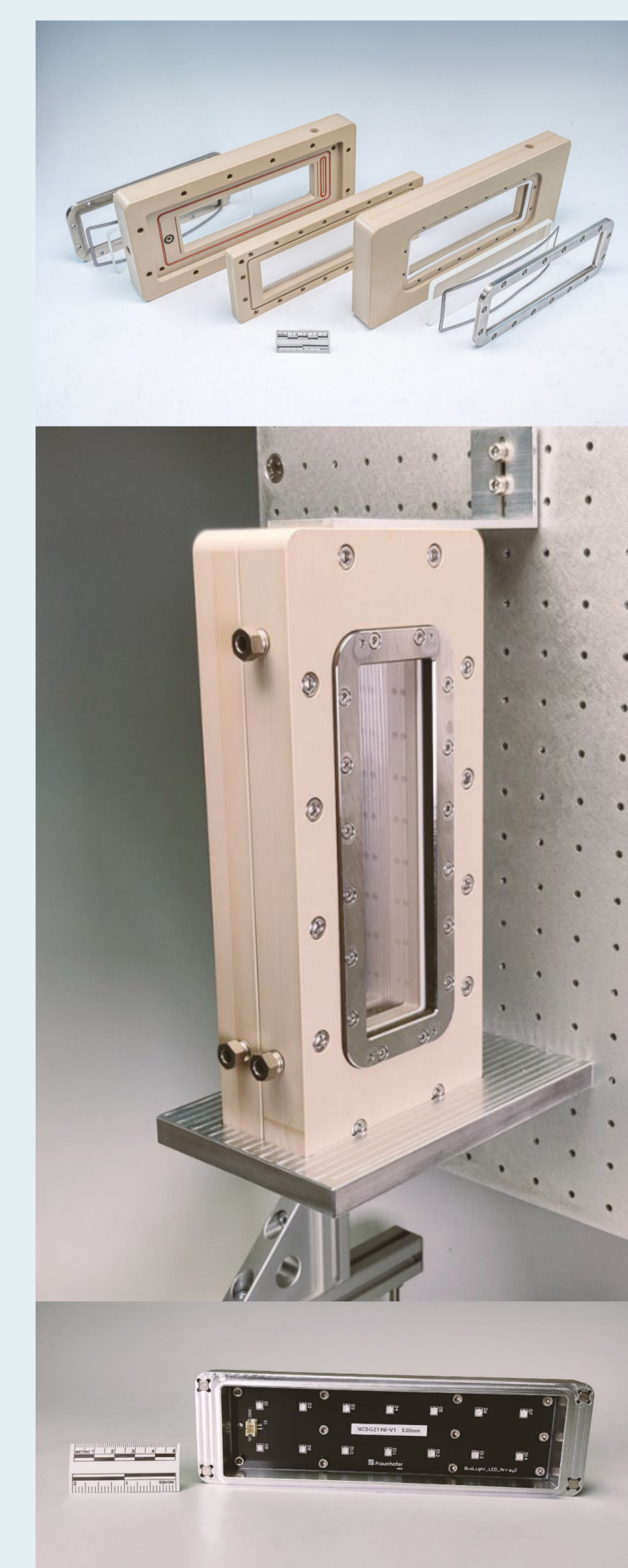
Figure 4: Disassembled FFMR with central frame carrying the PP foil (top); assembled FFMR installed as single reactor module (middle); high-power LED array with magnets for easy attachment to the reactor housing.
